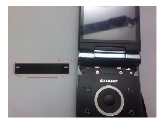
Now try to remove rest of bottom cover, start with tool on some corner (maybe bottom is better), then slide down (or up) on side.
