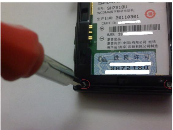
Remove plastic cover above keyboard, its not difficult to remove use nails or flat screwdriver and unscrew next 2 screws.
