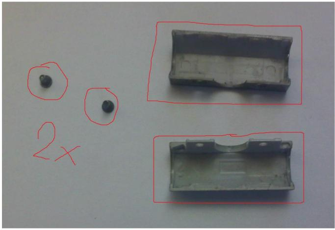
There should be 2 screws which holding flip mechanism. (I had only one, why?). When you removing this screws very carefully or you can damage display cable.
