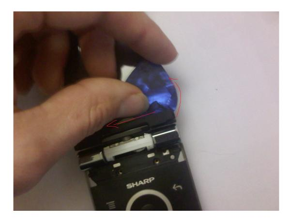
There are two screws and at the bottom side of plastics is some silicone (glue) which holding this pieces.
