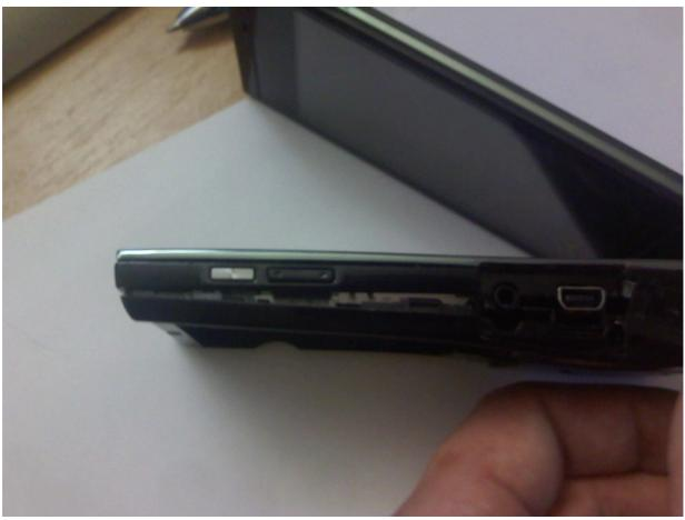
At this point very **carefully** remove whole back par, look out about flex and wires!
