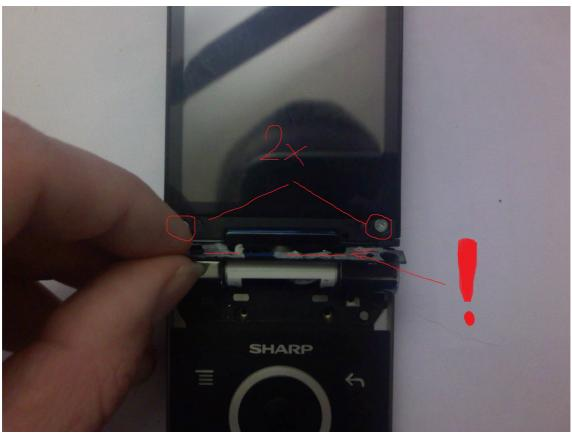
I heaved left upper corner and slide down for remove upper cover of display, the same other side.
