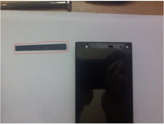
I used flat screwdriver to heave right corner of plastic cover under display, and tool which slide to remove this cover.
