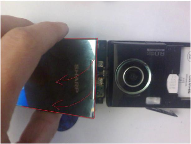
Don't lose small piece of rubber at bottom part of display.
